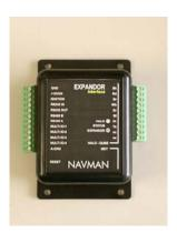
Navman provides this unit as a standard means of interface to vehicle peripheral devices in our CDMA Qube. It provides functionality if required such as analogue and digital inputs/outputs along with the serial ports RS232 and RS485. A PDA, temperature or weight monitoring are just some examples of peripherals that can be monitored using these serial ports.
