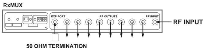
The Expansion Port can be used to expand the initial eight (8) RF outputs up to sixteen (16) RF outputs, all of equal net gain, through the use of an Expansion Multicoupler. If the Expansion Port is not used it should be fitted with a 50 ohm termination.
