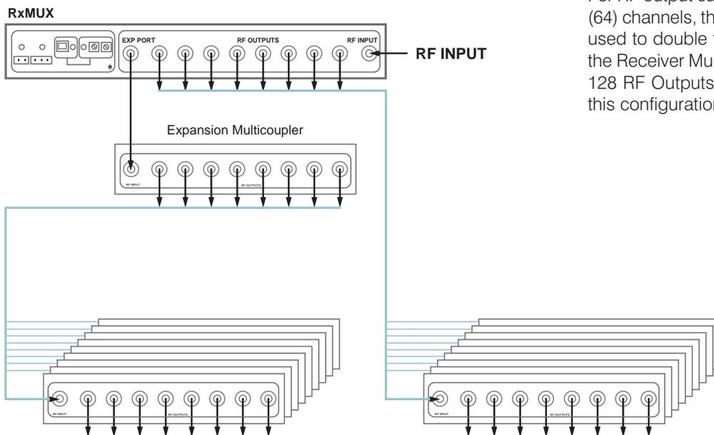
For RF output capacities above sixteen (16) channels, the Expansion Port should be terminated and multiple Expansion Multicouplers connected to the Receiver Multicoupler RF Outputs. Up to sixty-four (64) RF Outputs can be provided through this process.
