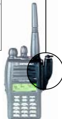
Accessory adaptor to be used with 3.5mm threaded range of audio accessories.
